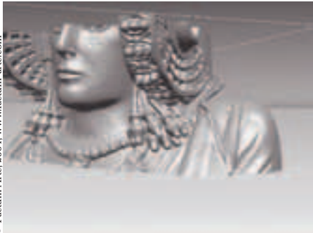
Data from the ModelMaker Scanner. In practice the best resolution achieved with the ModelMaker was 100 microns along the scanning line and 250 microns between lines.
