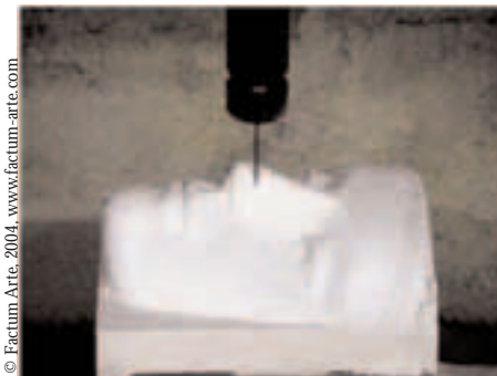
Each stage of the routing is done with increasingly fine cutting tools. The final pass is with a conical tool with a tip of 100 microns.
