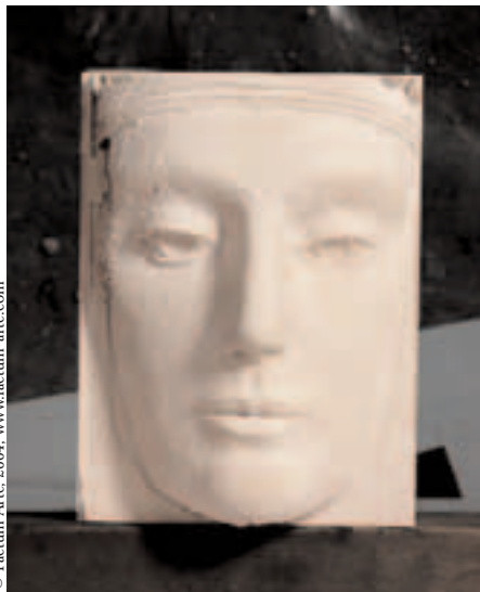
Routed face from the unmeshed Seti Scanner data. The routing was carried out by Delcam UK using a complex routing strategy with a final cut of 100 microns
