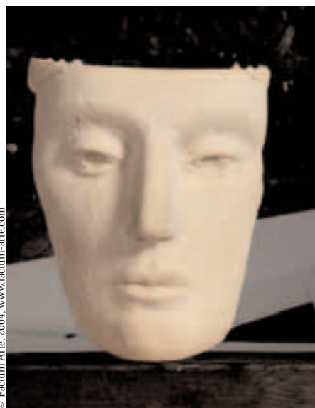
Z Corp print of the face from the meshed Minolta data. The Z corp print was made in 100 micron layers but compared to the milled data from the Seti Scanner the surface lacks detail and has the appearance of a sucked sweet.
