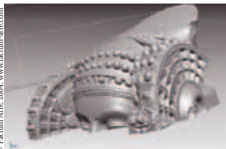
Data from the ModelMaker Scanner. In practice the best resolution achieved with the ModelMaker was 100 microns along the scanning line and 250 microns between lines.
