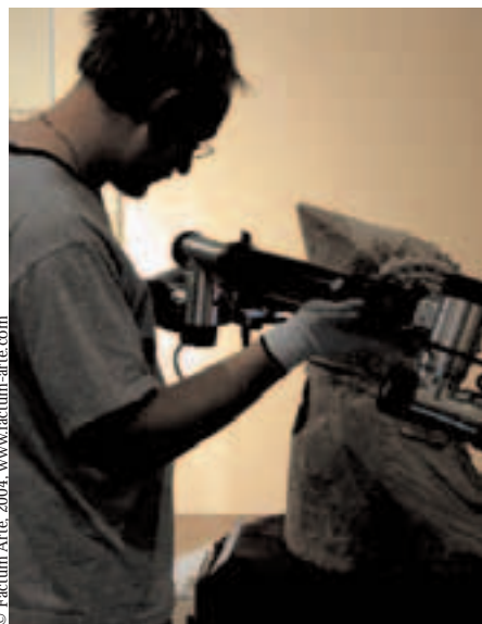
The ModelMaker Scanner recording the surface of The Dama de Elche in the Museo Arqueológico Nacional, Madrid.
