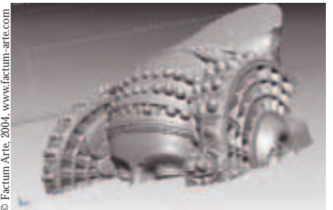
Data from the ModelMaker Scanner. In practice the best resolution achieved with the ModelMaker was 100 microns along the scanning line and 250 microns between lines.
