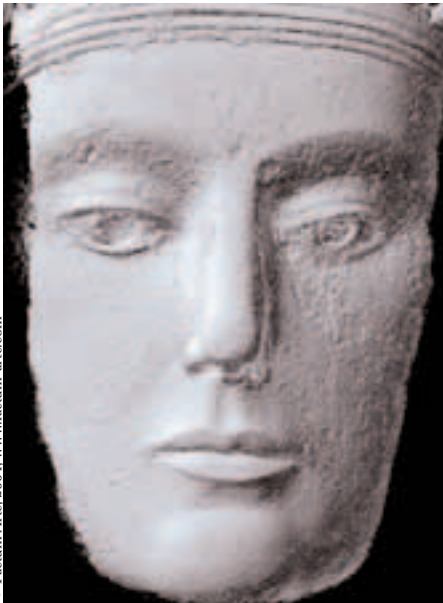
Data from the Seti Scanner. The data is made up of points of 3D information positioned on a 100 micron grid and requires no meshing or post processing
