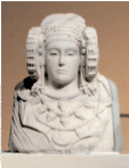
The finished Z Corp 3D print from the ModelMaker data. The data was output in 3 sections in layers of 100 microns. The two horizontal joints are clearly visible due to slight changes in colour of each section.
